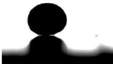
Fig. 1. Round particles made by the dropping method
