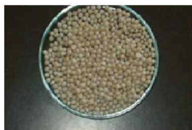
Fig. 1. Round particles made by the dropping method
