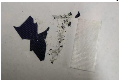
Figure 3.2: Solar cells, Glass, and residual obtained from tube furnace after the experiment Experimental Work:
