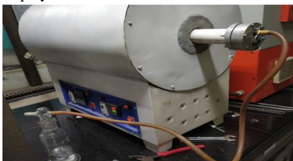
Figure 3.1: Tube Furnace setup with bubbler (Courtesy PM, lab IITB)
