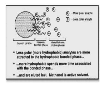
Figure 1.4.1: Reverse Phase Mechanism in HPLC
