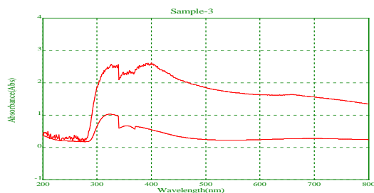
Fig 2: UV-Vis absorption spectra of copper nanoparticles using S. acidum
