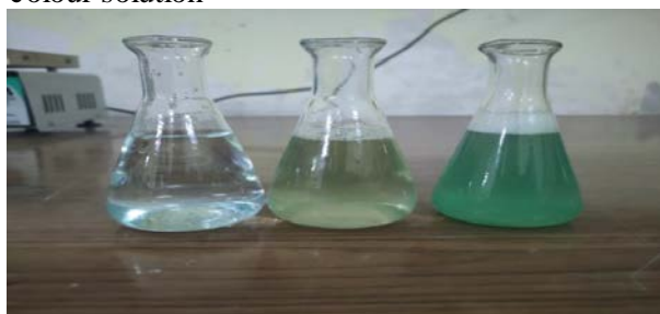
Fig 1: a) \text{CuSO}_4 solution; b) \text{CuSO}_4 and plant extract; c) CuO formed nanoparticles
